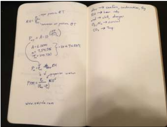
Notes on calculating the proportion of water molecules in the air from temperature, pressure, and relative humidity. On the right, plans for the macro-feedback descriptors.
